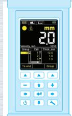
The mode is used for thickness measurement of the object on-the-spot along with display of the previously saved resulted (groups - cells in the groups - results) on the instrument's screen.
