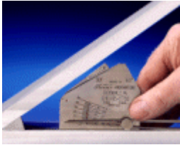
Checking Angle of Vertical Member
