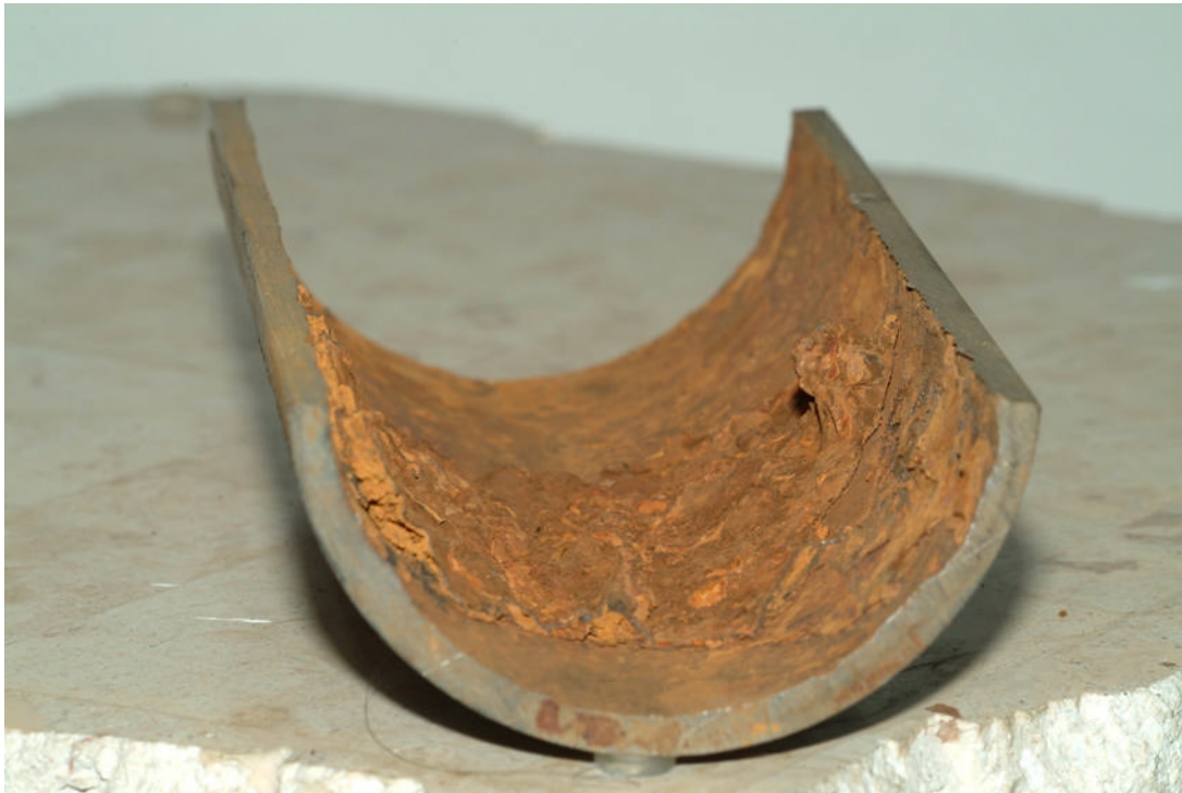
Figure 2. Corrosion Scaling in Fire Sprinkler Pipe
